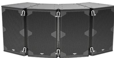
The FR-X rigging system allows assembling a horizontal or vertical array with constant curvature. Coupling between traditional horns causes a lot of comb effects resulting in poor sound projection and coherence in the space due to bad coupling between cabinets.
